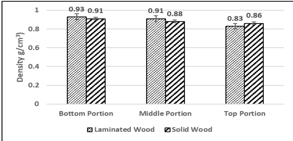
Figure 2: Density for laminated wood and solid wood at different height portion
