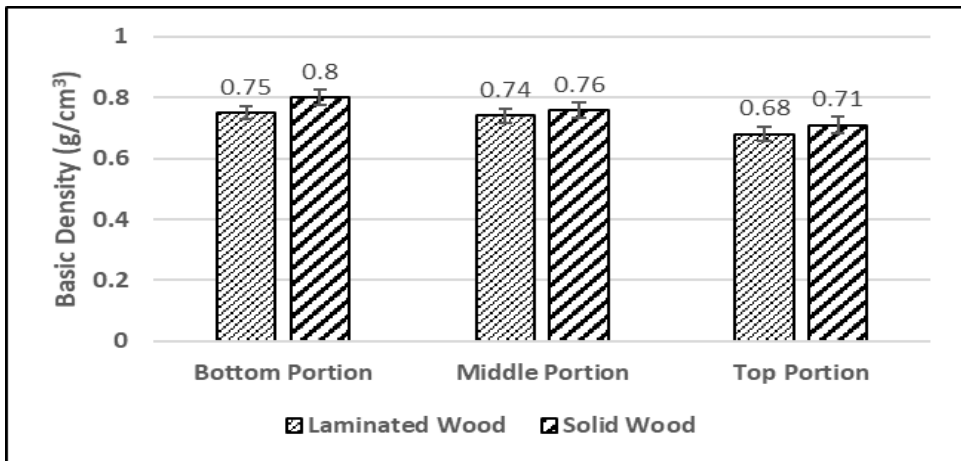
Figure 3: Basic density for laminated wood and solid wood at different height portions
