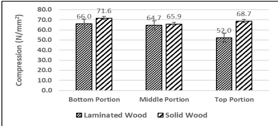
Figure 6: Compression test on solid wood and laminated wood at different height portions.
